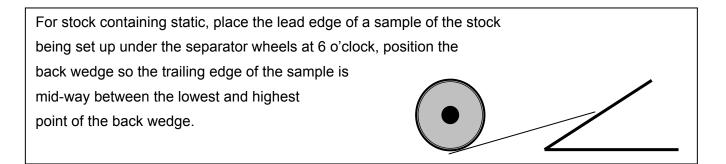
**Note:** These are basic starting points for a set-up. Further adjustments may be required.
