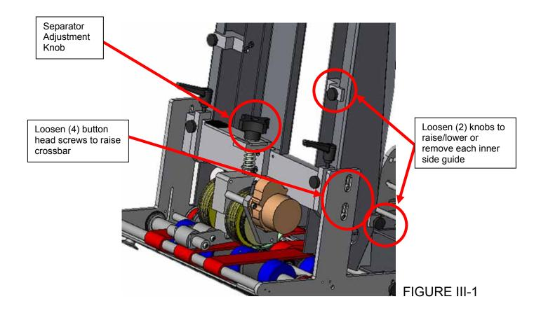
2. Raise both separator wheels by turning the adjustment knob atop separator assembly in a clockwise direction, see figure III-1.
